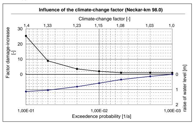
**Figure 1:** Influence of the climate-change factor on water depths and potential flood damages in the municipality of Offenau (Neckar km 98.0).
